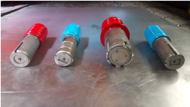
Fig. 6 Example of color code for the shape of the punching machine tools.
