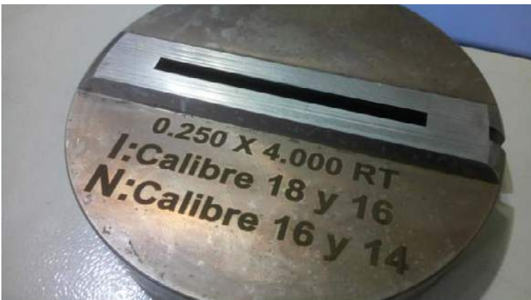
Fig. 7b Final state of the tool with the engraving of technical specifications applied to be identified easily.
