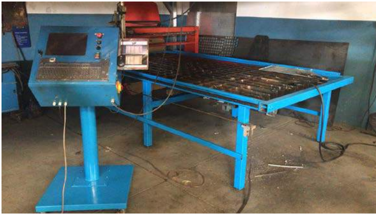
Fig. 14 Previous plasma cutting machine with height of 1 meter and without torch height control.
